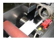
Pneumatically actuated perforation wheels are used for U-board applications.
