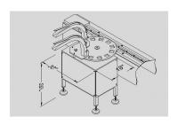
Vertical Disk Feeders minimize floor space requirements and are typically fed with fully automatic distribution systems
