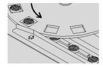
Horizontal disk presents product to wrapper flights at proper spacing and speed for smooth, gentle transfer
