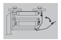
Hinged guards and cantilevered design provide access for maintenance and sanitation.
