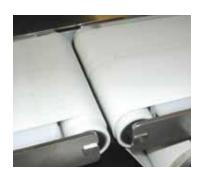
Frames are laser cut to allow for easy removal of end rollers.
