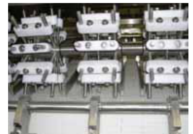
Spring loaded release shaft self-clears partial products.
