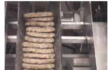
Product is shingle stacked by count in multiple lanes. Slugs are simultaneously released to the rodded conveyor positioned below.
