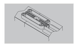
Contoured side belts keep leading and trailing products upright during transfer into the spring loaded wrapper flights.
