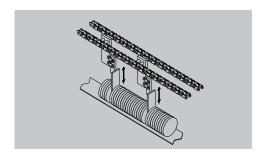
Floating measuring pin gently enters a continuous lane of on-edge product without causing damage.
